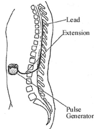
The permanent spinal cord stimulator is a patient controllable pacemaker type of generator that is implanted under the skin above the hip and connected to leads placed into the epidural space. The electrodes on the leads stimulate the spine at a higher frequency than do incoming pain nerve signals, thereby causing the spine to filter out most of the incoming pain. Different stimulation patterns and electrodes may be activated to treat different types of pain.
